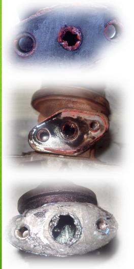
Effects of using gasket sealant paste on turbocharger:
